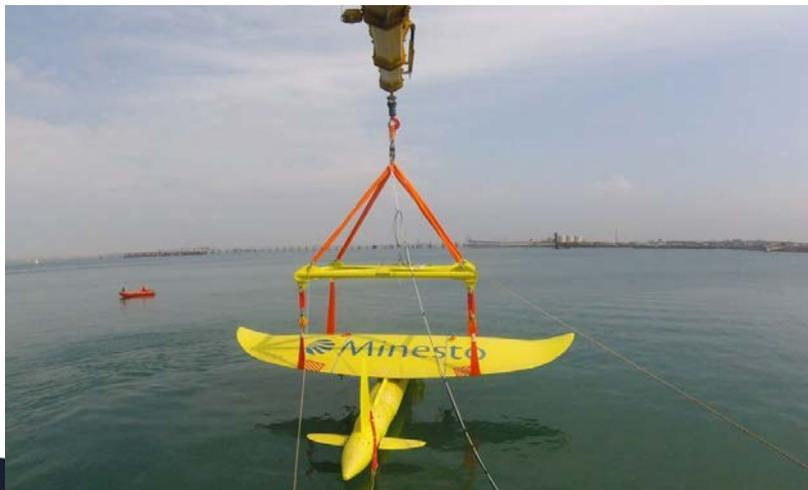
The first **0.5MW** utility-scale system of **Minesto's** patented **Deep Green** technology has been commissioned at the Holyhead Deep site off the coast of North Wales, (October, 2018)
