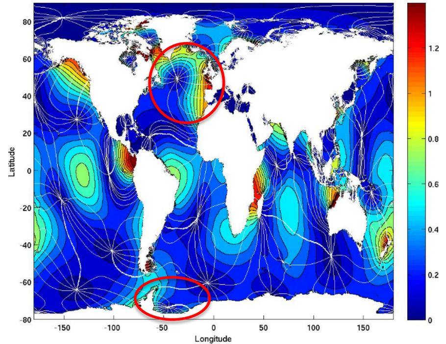
More accurate M2 co-tidal chart obtained after updating the model bathymetry around Antarctica using the BedMap2 data set, including effects of ice
